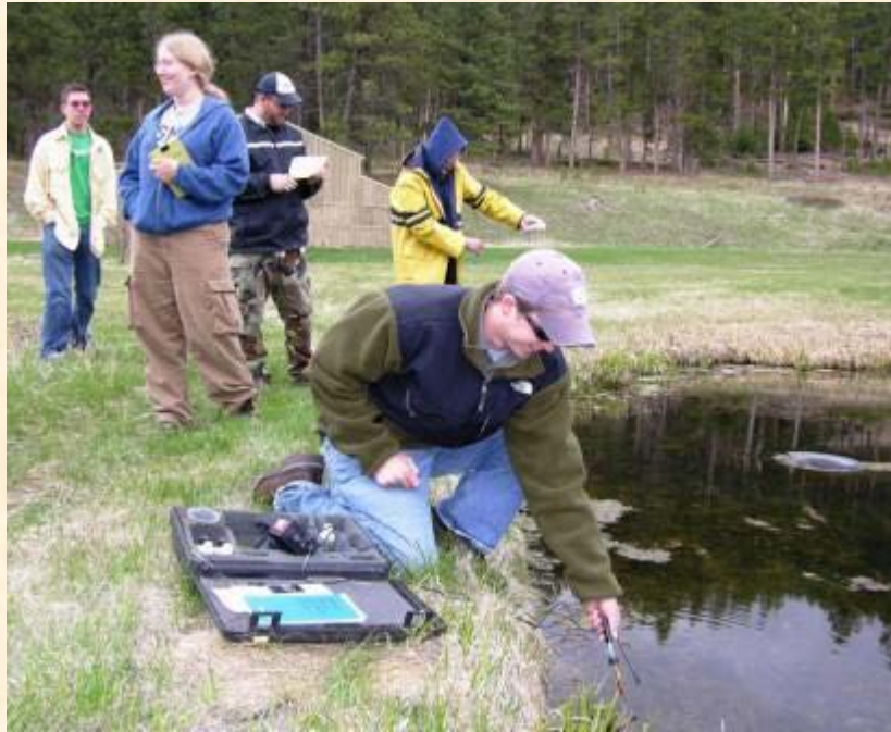
Photo 1—Dr. Arden Davis’ Geochemistry class from the South Dakota School of Mines and Technology sample water on May 5 th , 2007. Josh Valder, one of the students in the class, is measuring the temperature and pH of the carbonate spring waters. The out-gassing of dissolved CO 2 changes the solubility of calcium carbonate (limestone) with distance from the springs creating travertine deposits and waterfalls.
